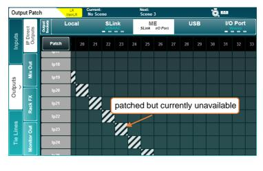
() All patching to a currently disconnected device will become active once the device is connected.
