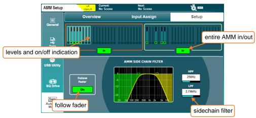
Like the '**Overview**' screen, this displays an overview of all AMM slots, with gain metering and indication of whether or not channels have AMM switched on.
