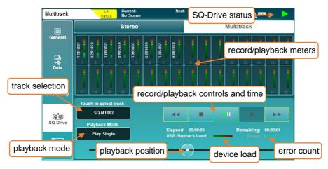
In 96kHz operation the top row of 16 meters is displayed with the bottom row greyed out. When the USB sample rate is set to 48kHz, all 32 meters are shown.
