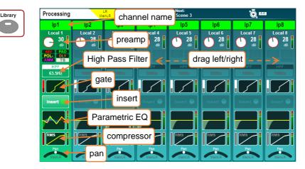
Press the 'Processing' screen key to display the processing 'bank view'.
