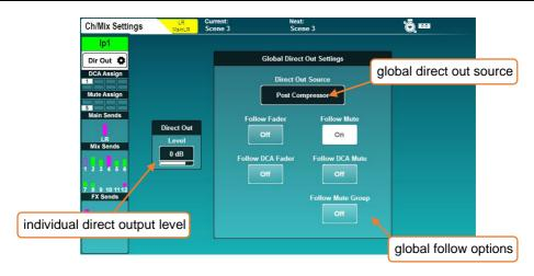
Touch the 'Dir Out' button on any input channel.
