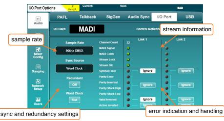
Information on the MADI stream for each Link is displayed to the right of the main settings, including error indication. If an error is detected on the stream, incoming audio will be muted, so an option to ignore these errors is provided for greater compatibility with third party equipment.
