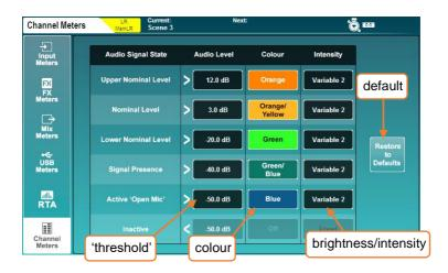
• Touch an 'Audio Level' value and adjust using the touchscreen rotary.
