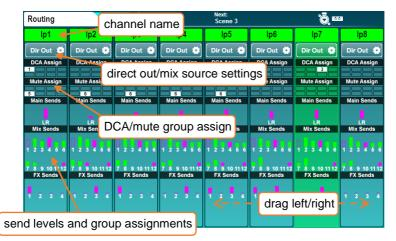
If a channel is assigned to a DCA or Mute group, this is shown with a filled, numbered icon.
