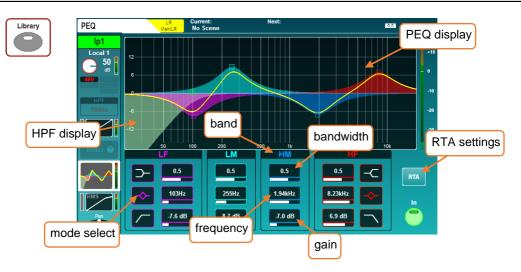
The PEQ can be switched in or out using the physical '**In**' key on the surface or with the on-screen '**In**' button.
