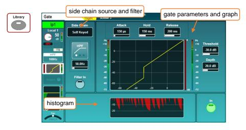
Switch the Gate in or out using either the on-screen '**In**' button or the physical Gate '**In**' key (to the left of the dedicated Gate threshold rotary).
