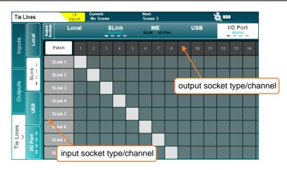
Tie lines are used to patch connections directly between source and destination points without using any of the channel processing, mixing or level control in the core.
