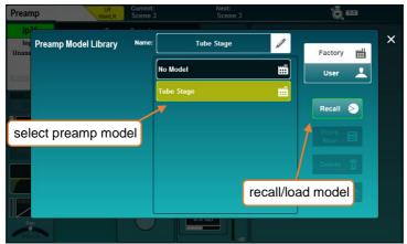
• Select a preamp preset, then press the 'Recall' button to load it.
