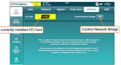
This screen shows information and settings for the option card which is currently connected. It also contains the '**Control Network Bridge**' switch.
