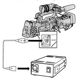
2 Turn on the power of the AC adapter, followed by setting the [POWER ON/OFF] switch of this unit to "ON".
