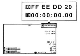
2 Select the display using the [TC DISPLAY] switch on the LCD monitor.
