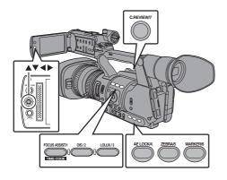
1 Assign functions to the buttons from the menu. Set items in [Main Menu] → [Camera Function] → [User Switch Set] → [USER1]-[USER7], [LCD KEY▲], [LCD KEY▶], [LCD KEY▼], [LCD KEY◄].
