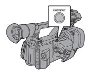
Press the button assigned with the "Clip Review" function during standby ("STBY" is displayed). Playback of the configured section starts.
