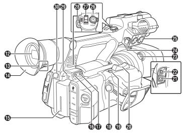
(B) [REC] Record Trigger Button Starts/stops recording.
