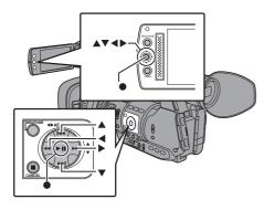
1 Select the following in [Spot Meter] of the [Main Menu] → [Camera Function] → [User Switch Set] menu.
