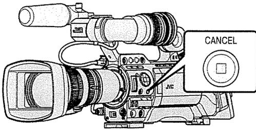
**1 While in the Camera mode (when the display screen appears), press and hold the [CANCEL] button for 5 seconds or longer.**
