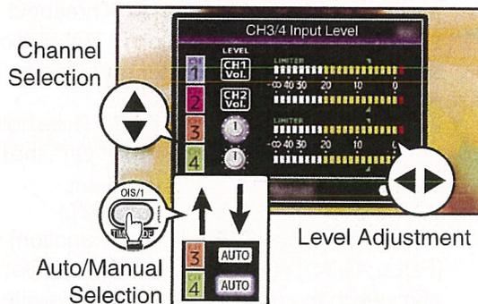
**3 Press the Set button (●) to end the adjustment.**
