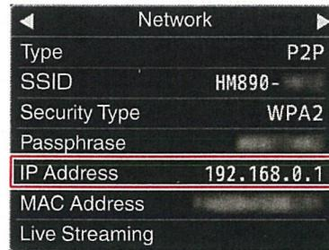
**2 Start up the web browser on the terminal you wish to connect to the camera recorder, and enter the [IP Address] in the address field.**
